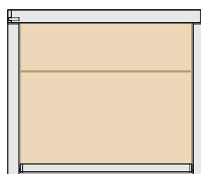
Transverse seam in the top third (on request, no surcharge)
